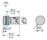
Support panel thickness: 1 to 6 mm/0.4 to 0.24 in. (metal), 2 to 6 mm/0.8 to 0.24 in. (plastic).
